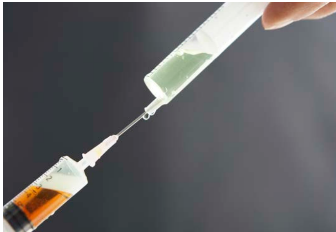
Fig. 54: Passing Chlorine dioxide gas into a saline solution using syringes
